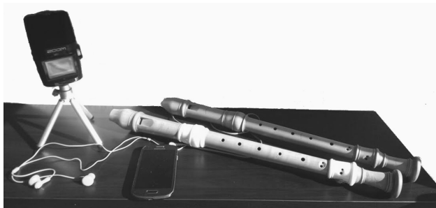
Figure 2. Apparatus for the experiment, showing (A) sound recorder, model ZOOM H2n, (B) phone with metronome app bestmetronome and headphones, (C) f-alto recorder at A=415Hz by Doris Kulossa, (D) f-alto recorder at A=440Hz by Ralf Netsch. Photo by Naomi Nordblom.
